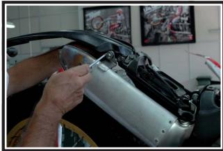
Remove the five rivets on the muffler terminal.
