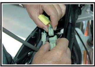
Disconnect the WHITE / GREEN cable from the clamp by using a screwdriver.
