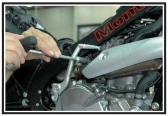
Remove the two screws (a) from the exhaust pipe to the cylinder.
