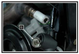
Remove the coil to take off the O<sub>2</sub> sensor cable
