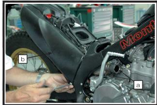
Replace the exhaust pipe manifold (a) with the new manifold (b) supplied in the kit.
