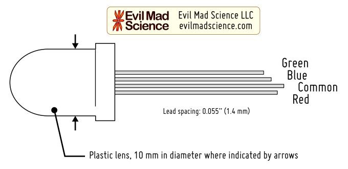
• Milky-white diffused lens gives wide viewing angle and excellent color mixing. Best lens choice for indoor viewing.
