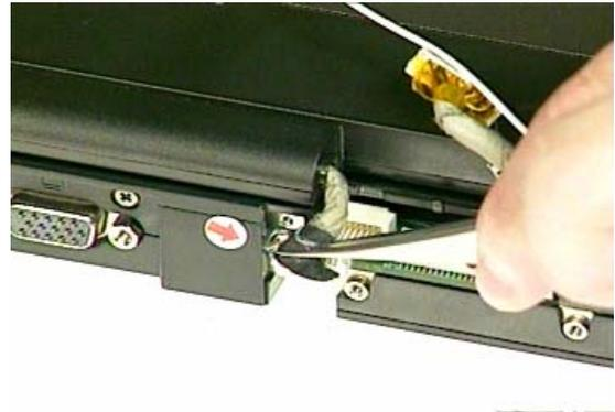
7. Remove 2 screws on both ends.
