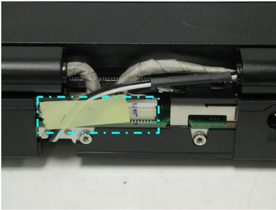
5. Remove 1 screw and disconnect the connector.
