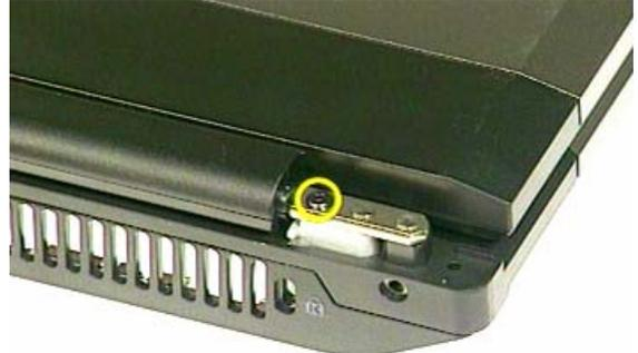
8. Remove the LCD module from system.
