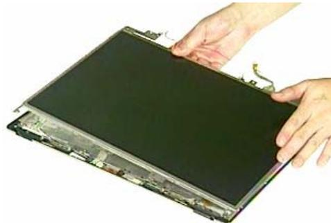
2. Finally, Remove 4 screws on the right LCD bracket, and 4 screws on the left side to disassemble LCD brackets.
