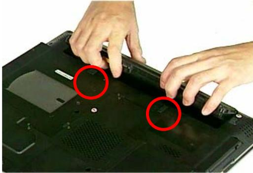
2. Slide the battery latch (No.1) to unlock and Firmly slide the other latch (No.2) to the top and remove the battery
