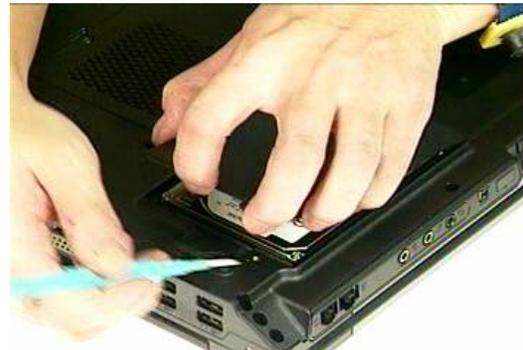
3. Push the metal plate with a screw driver and pull the ODD out.
