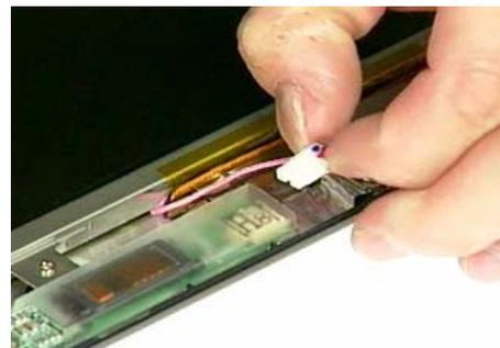
4. Disconnect inverter cable and take away the inverter board.
