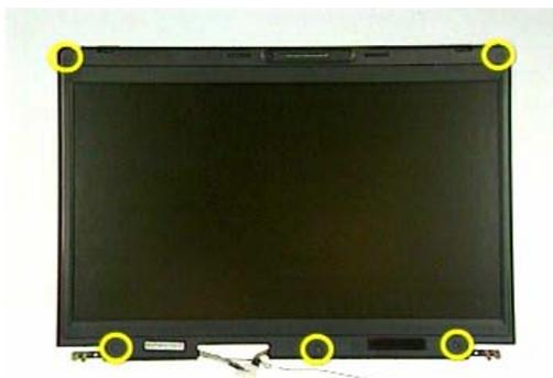
2. Prying the inside edges of the bezel, then separate it from LCD back cover and take LCD front bezel away.
